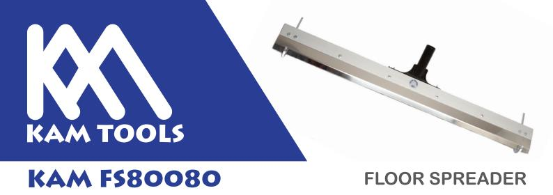
Our **KAM F\$80080** Floor Spreader is an adjustable heavy-duty leveller for the application of flowable overlay materials applied in excess of 4mm thick. The 800mm long stainless steel levelling blade features hard-wearing adjustable steel skis at each end that provide fine adjustments from as little as 0mm to as much as 50mm thick.
